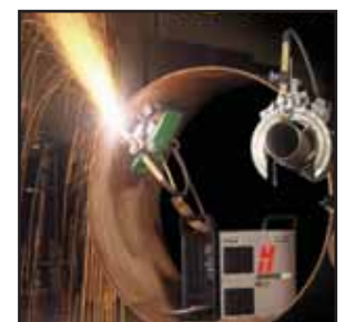
Pipe and bevel cutting
