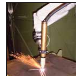
Robotic 3-dimensional cutting
